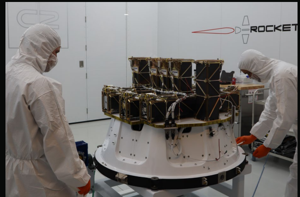
◉ 'ELANA-19' PAYLOAD INTEGRATION ON THE KICK STAGE | 2018
