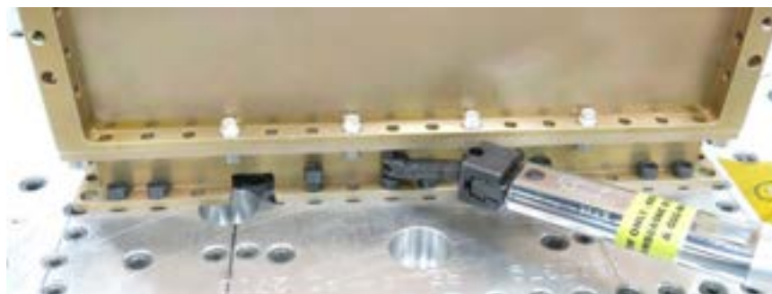
Figure 20-3: Using reduced clicker head wrench to torque fasteners via -Z face
