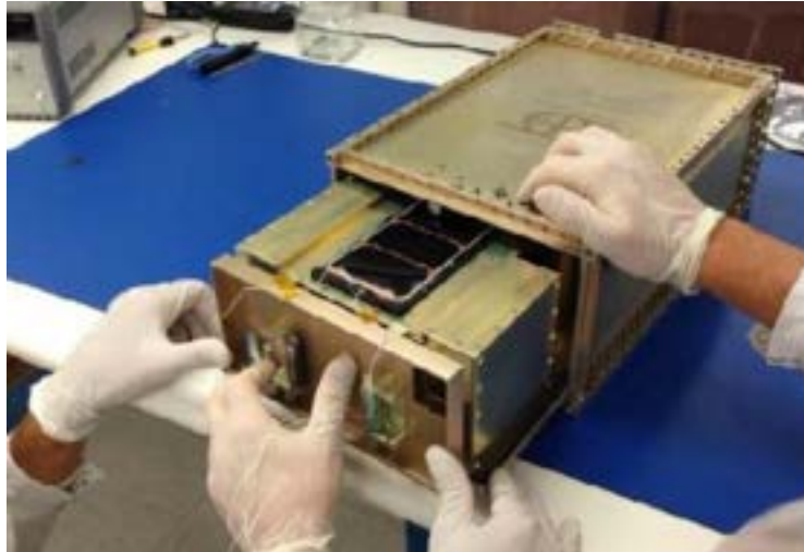
Figure 20-1: Installing 6U payload in CSD
