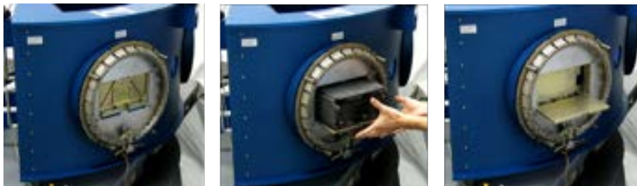
Figure 24-1: 6U payload deploying through ESPA port. CSD mounted directly via +Z face.
