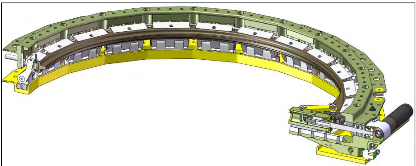
Figure 7-6: The Leaves disengaged during deployment, (section view)
