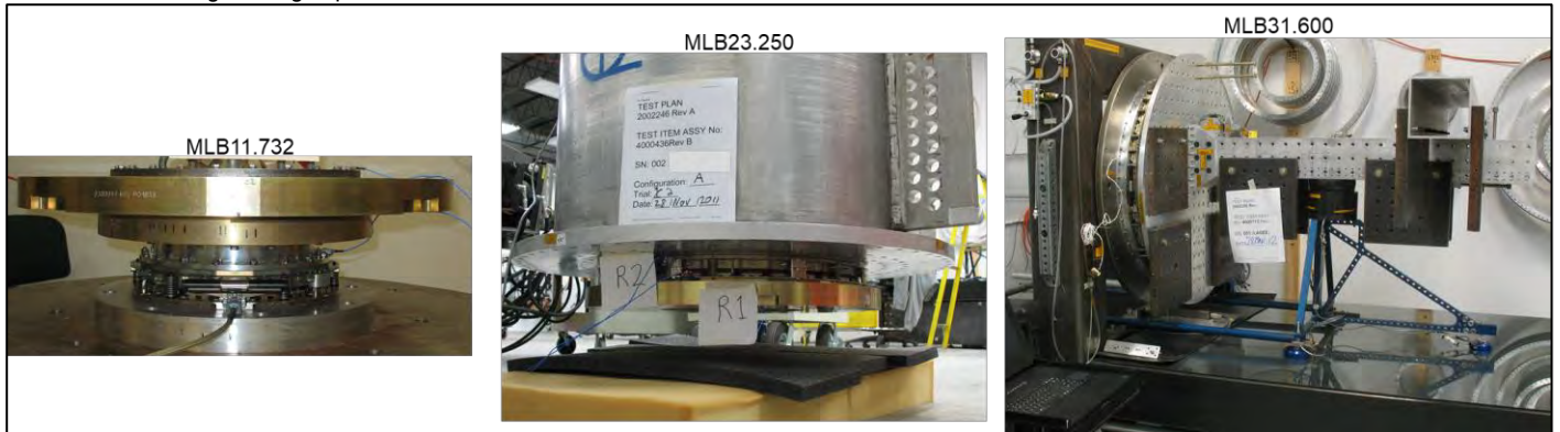
Figure 10-3: Test configurations for MLB generated shock
