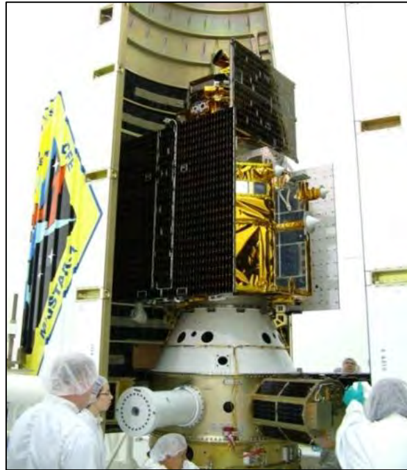
Figure 2-7: MLBs on ESPA (STP-1) on an Atlas V
