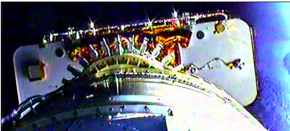
Figure 2-2: Two of NASA's lunar GRAIL satellites separate from a Delta II in 2011 using 2X MLB19.848
